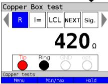
In this example, a loop resistance of  $420 \Omega$  is measured.
