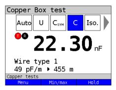
In this example, a capacitance of approx. 22.30 nF is measured between Tip/Ring. On the basis of the values stored under wire type 1, this corresponds to a 455 m line
