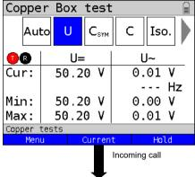
In this example the Copper Box is connected so as to measure the voltage of an POTS access.
