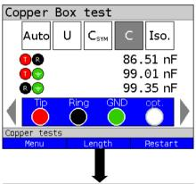
In this example, a capacitance of approx. 86 nF is measured between Tip/Ring. For a capacitance of approx. 49 nF/km, this value indicates that the line is approx. 1.77 km long.
