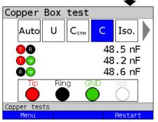
In this example, a capacitance of approx. 48 nF is measured between each of the sockets Tip/Ring and Ground. For a specific capacitance of approx. 50 nF/km, this value indicates that the line is approx. 1 km long and open.
