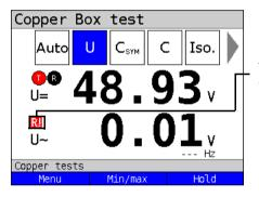
The example here shows a low-ohm (loaded) measurement.
