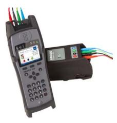
The box is connected to the ARGUS tester simply via the USB host interface. You can select the box and perform all measurements easily and rapidly via the ARGUS graphical user interface.
