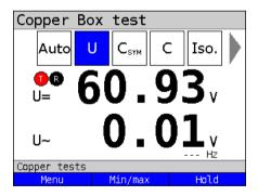
The measured voltage of 60.93 V could indicate an POTS access
