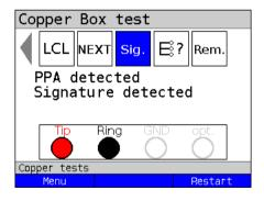
In this example, a PPA and a signature circuit between Tip and Ring were detected.
