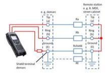
Values Ra, Rb and RE are not measured directly, but instead are calculated from three individual measurements (Rab, RaE, RbE). The caculated values are then used in determining symmetry.
