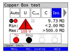
Fast "Isolation resistance measurement", e. g. of all pins at the demarcation point with respect to each other and earth.
