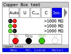
The example shows the measurement of a resistance between Tip/Ring, Tip/ Ground and Ring/Ground of >1000 M $\Omega$ . This indicates that the line is not damaged. Depending on the requirement, a value of e.g >300 M $\Omega$  is considered good. Values <300 M $\Omega$  and >5 M $\Omega$  should be examined more closely. Values under 5 M $\Omega$  indicate an isolation fault.
