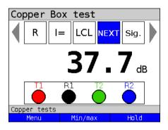
However, a value >37 dB (as in this example 37.7 dB) considered sufficient. The crosstalk to the adjacent line is tolerable.
