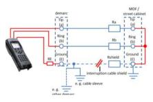
2. Measureing site, e. g. demarcation point: The demarcation point is not earthed. The cable shield is interrupted at the site shown in the illustration. However, the resistance symmetry measurement can still work if the cable shield at the demarcation point is connected to one of the earthing points shown in the picture. However, the RE measurement is not Rshield, as the shield can have an ground potential of varying quality due to the lead sleeve in the ground (obsolete constuc-
