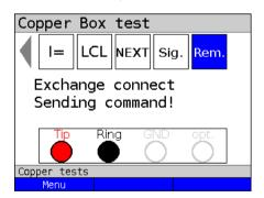
The command "Exchange connect" is sent to the remote unit.
