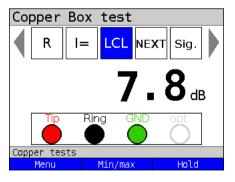
If a value <40 dB is measured, or even 7.8 dB as in this example, Tip or Ring may be shorted to Ground.
