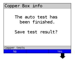
When the auto test is complete, the device automatically outouts a message and prompts you to save the results. After saving, ARGUS automatically switches to the view of the saved measured values
