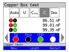
In this example, a capacitance of approx. 86.51 nF is measured between the sockets Tip/Ring.
