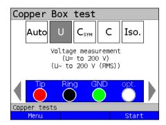
In this example, sockets Tip, Ring and GND are selected.
