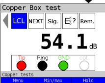
In this example, an asymmetry attenuation of 54.1 dB is measured.
